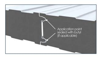
In the case of negative temperature chambers, it will be necessary to seal the interior joint between panels with butyl (or equivalent product) at least on the face with the highest temperature in order to avoid the permeability of water vapor through the joint.
