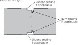
This panel is not indicated for use as a freezing chamber (T>0°C) without adequate treatment of the joints during assembly. In the case of the panel in the ceiling position, it may be damaged when walking over it during the installation or maintenance process. Therefore, the applied loads must be in accordance with what is indicated in the technical sheet and it is also advisable to place protection in the passage area to avoid delaminations.
