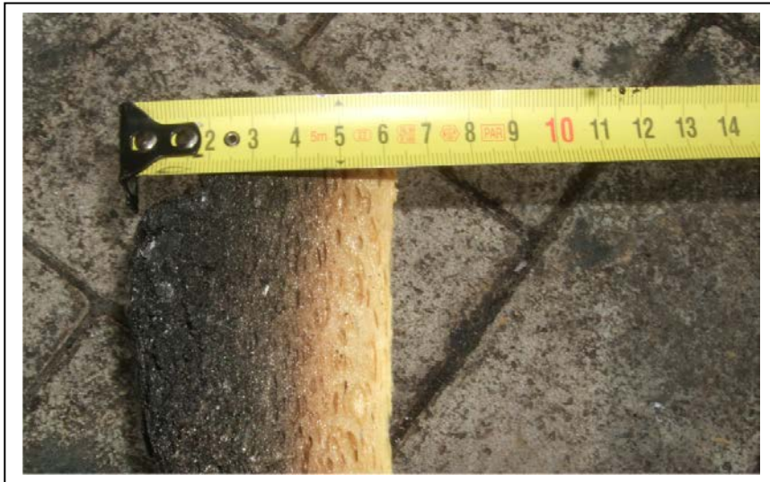
Figure 5 – sample of PIR core removed from cladding panel at location of estimated peak incident radiative heat flux.
