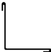
Flashing Inner corner angle
